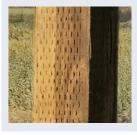
is a heartwood penetration requirement (even for permeable species such as pine). Mechanical incising of the surface is now used widely to help achieve the desired penetration.
