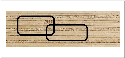
Products made of rotary peeled veneers are more homogeneous than solid wood due to dispersion of natural defects such as knots.
