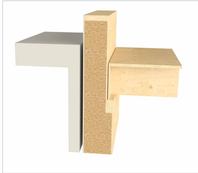
Load-bearing wall, lintel support
