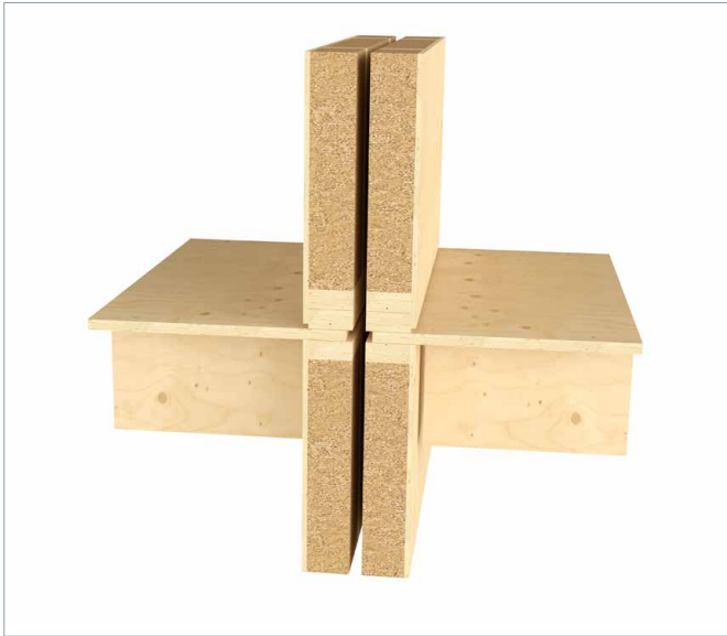
Load-bearing separation wall, top-plate support
