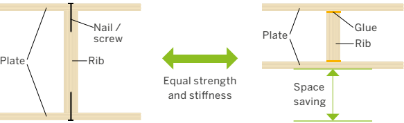
Depth savings between mechanically fastened elements and Kerto-Ripa glued elements
