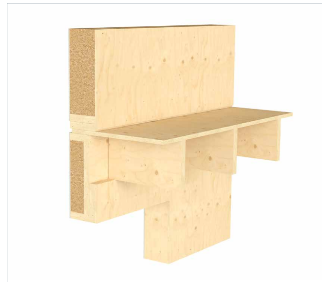
Load-bearing separation wall, lintel support over wall opening
