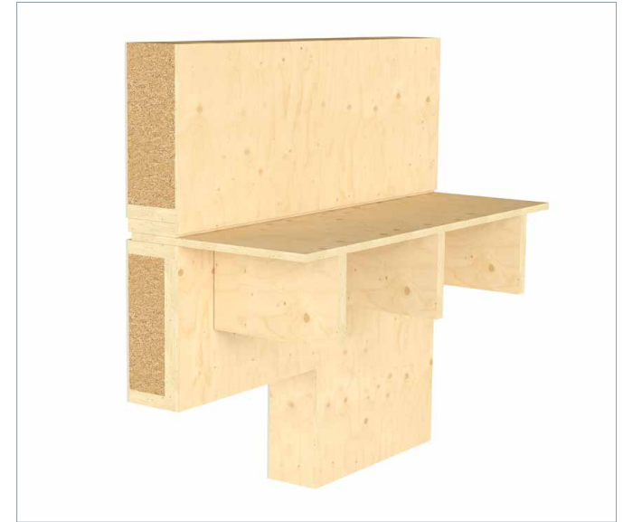
Load-bearing wall, top-plate support over wall opening
