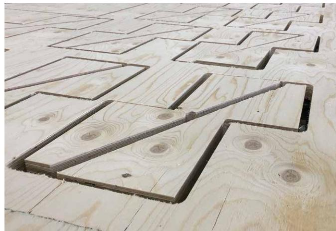
Figure 3. CNC machined Kerto LVL
