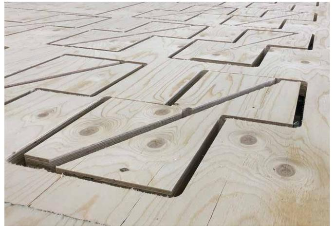
Figure 3. CNC machined Kerto LVL
