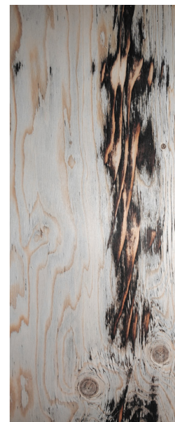
Figure 6. Front side, sanded through
