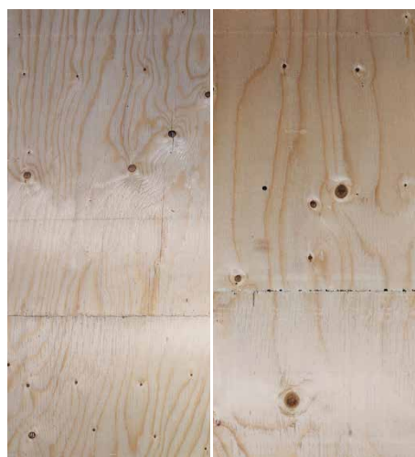
Figure 2. Front side, unsanded, light colour glue in scarf-joints
