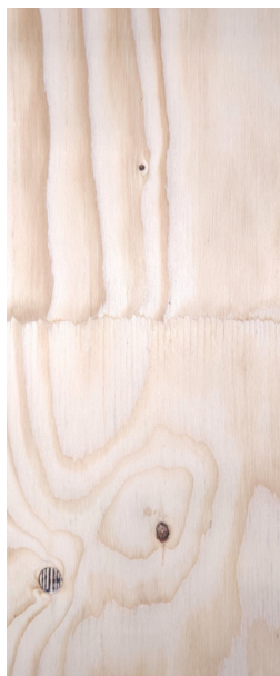
Figure 4. Front side, optical sanded, light colour glue in scarf-joints
