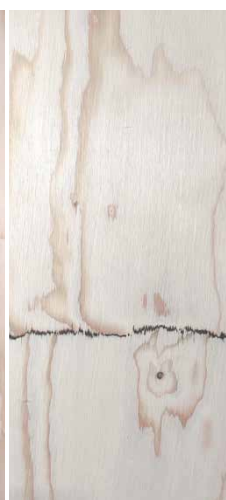
Figure 5. Reverse side, optically sanded, dark brown glue in scarf-joints
