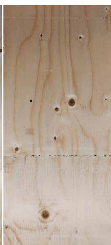
Figure 3. Reverse side, unsanded, dark brown glue in scarf-joints
