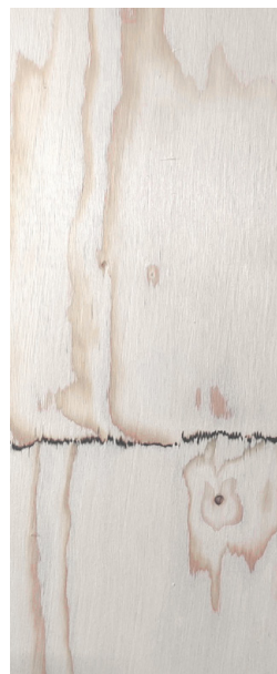
Figure 5. Reverse side, optical sanded, dark brown glue in scarf-joints
