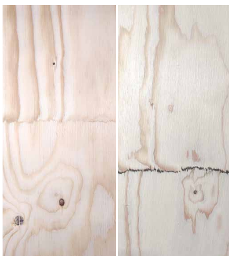
Figure 4. Front side, optically sanded, light colour glue in scarf-joints
