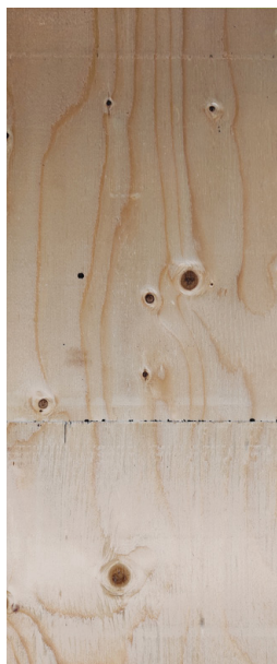
Figure 3. Reverse side, unsanded, dark brown glue in scarf-joints
