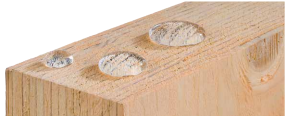
Figure 4. Water droplets on WeatherGuard treated Kerto LVL
