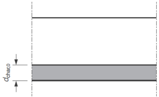
Figure 1: One-dimensional charring of wide cross section when fire exposure is on one side (Source: EN 1995-1-2).
