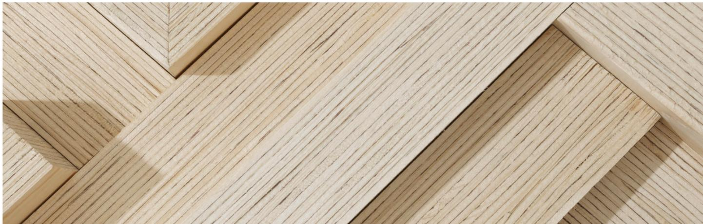
Kerto® LVL surfaces can be further treated with standard paints, lacquers, vanishes and protection treatments suitable to wood products. Surface treatments improve the properties of Kerto LVL without affecting the strength and stiffness properties. Compatibility of the surface treatments should be confirmed from the treatment provider. Surface treatments provided by Metsä Wood are presented in Kerto LVL Manual - Further processing.
