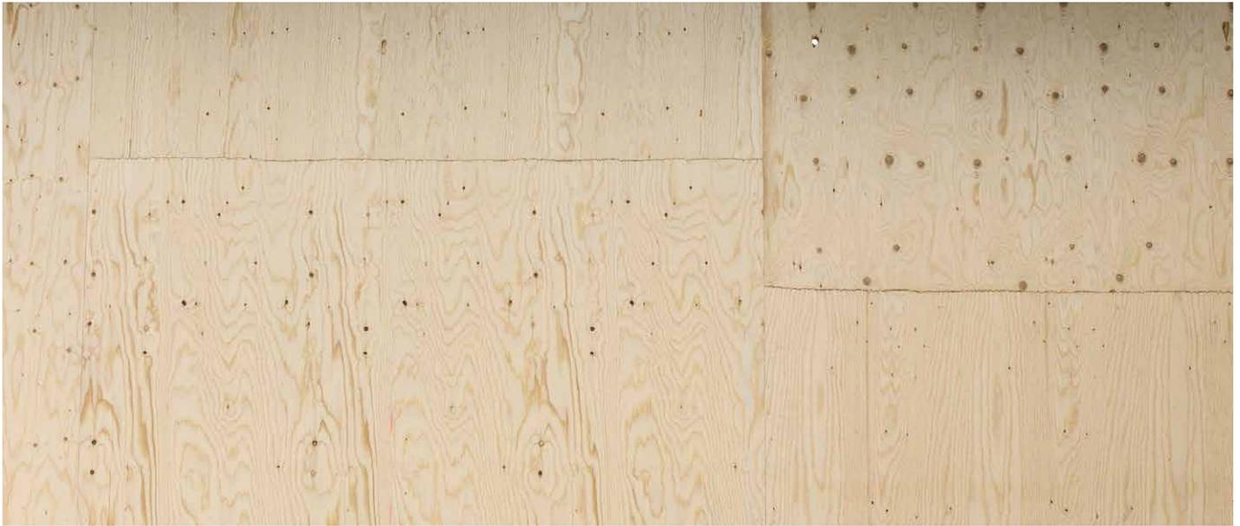
Kerto LVL surface quality. Metsä Wood provides the half-lap panels sanded on both sides.
