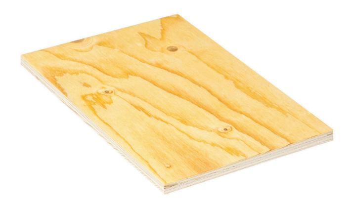
Metsä Wood Spruce FireResist is a surface impregnated softwood plywood with enhanced fire performance. The European reaction to fire classification for Spruce FireResist is B (according to EN 13501-1). The product is suitable for interior applications, and it must be protected from weather exposure at all times.
