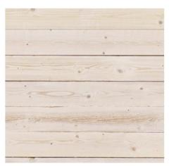
Small size and amount knot quality. On edges only small knots, often almost knotless.
