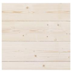
Best knot quality. Majority sound knots, dry knots 50% of sound knot side. No bark ringed knots allowed.
