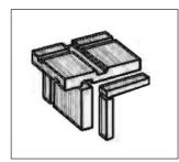
A FIRE LINING is made with rebated channels along the OUTSIDE of the set. These are for INTUMESCENT STRIPS that need to be installed prior to the lining being fixed into position. These strips will swell when exposed to heat and provide a vital barrier against heat and smoke transfer.
