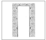
Using shims, blocks or wedges, secure in place the lining and make sure the HEADER is level. Use a spirit level.
