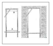
Stabilise the lining by temporarily fixing two pieces of scrap timber as shown, make sure dimension A is EXACTLY the same as B. This is IMPORTANT.
