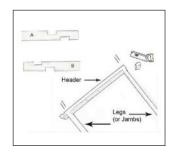
Flip the HEADER so that the required rebates are facing downwards, this depends on the width of the door. Fit the LEGS by way of four wood screws. Pilot-drill the holes first. Then, saw off any excess wood from the HEADER so that it fits in the doorway aperture.
