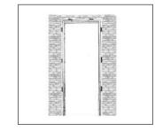
Making sure the frame stays straight, level and perfectly upright, fix the frame to the wall by way of 100mm screws. Frame fixings may be required depending on the material you are fixing to.
