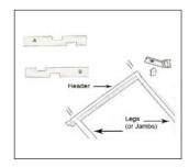
Flip the HEADER so that the required re-bates are facing downwards, this depends on the width of the door.
