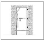
Using shims, blocks or wedges, secure in place the lining and make sure the HEADER is level. Use a spirit level.
