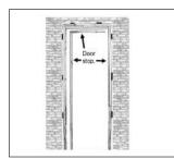
The door stops can be fitted AFTER the door has been hung, it is much easier to locate them perfectly this way. They can be pinned into place.
