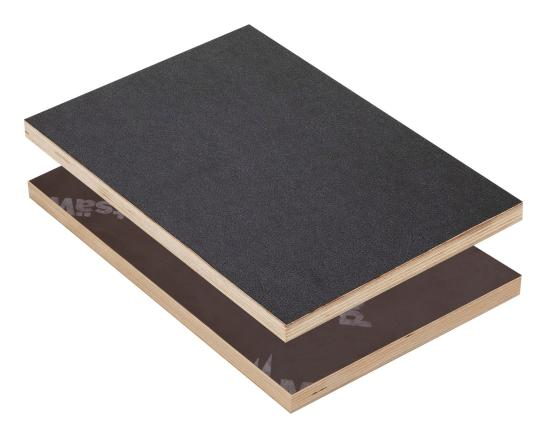
Metsä Wood DURAForm is a high performance formwork panel choice for smooth surfaced concrete elements. Metsä Wood DURAForm plywood has a special treatment to resist the surface rippling that ensures smooth high quality concrete finish from the first pour. Metsä Wood DURAForm panel surface is a multi-material composite that is harder and more scratch and wear-resistant than standard formwork panels.
